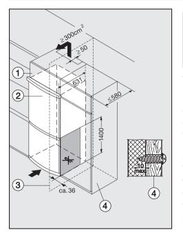
The appliance can be installed in a kitchen run. To match the height of the rest of the kitchen, the appliance can be fitted with a suitable top box ①.
